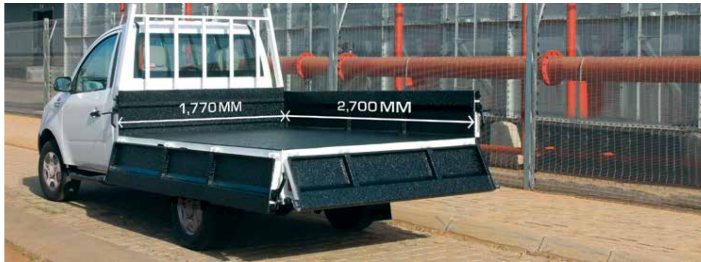
Above: The load box on the Genio Long provides over 1m 2 than the standard dropside
